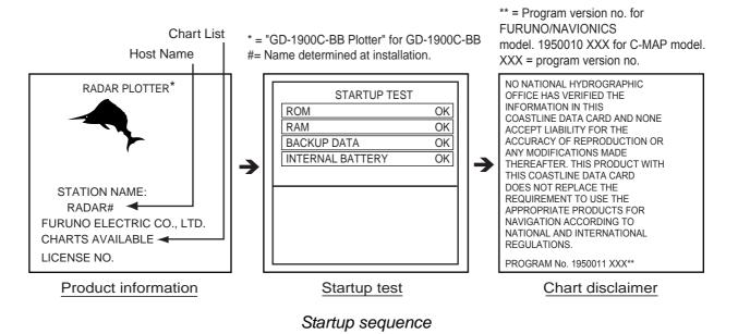
For start up with the radar display, the magnetron takes from one minute to two minutes and thirty seconds (depending or radar model) to warm up before the radar can be operated. The time remaining for warming up the magnetron is counted down at the center of the display.
